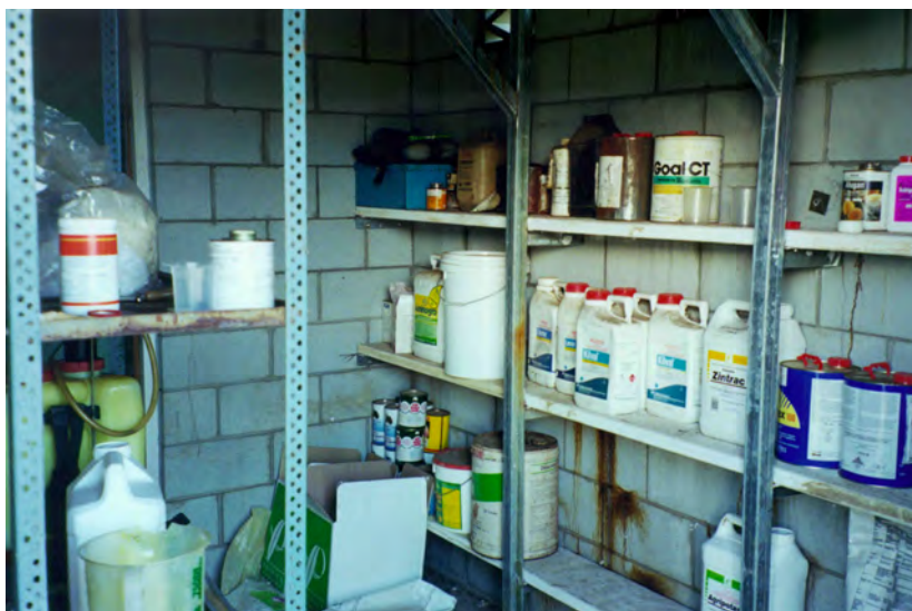
Figure 11. Chemicals must be stored in a well lit, sound and secure structure, with only authorised people allowed access.
