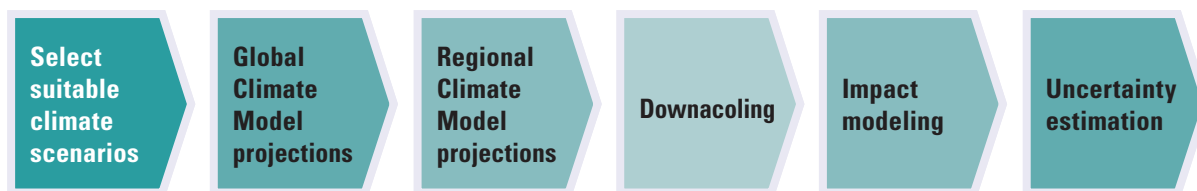
Figure 3.1 Proposed climate projection process for landslide risk assessment at a river basin scale
